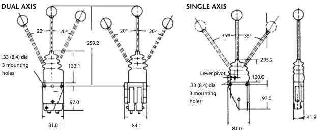
Single Axis systems consist of a control head, a cable of suitable length and a bonnet-type connection kit for each valve. Specify the correct cable length and appropriate conversion kit.
