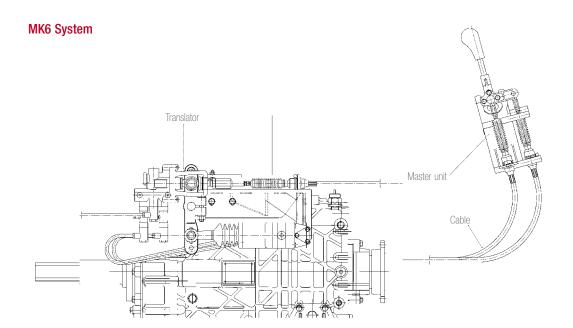
The MK6 System is composed of three main components.
