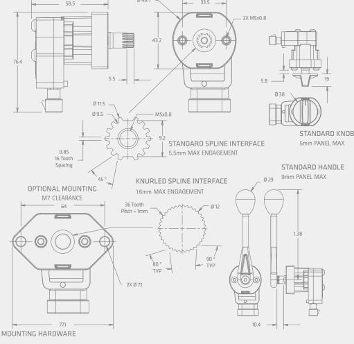
Standard Mounting: M5 x 0.8 x 30 Pan Head screws recommended.
